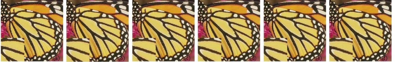
Fig. 6. Visual comparisons of the super-resolution results of our SMSR framework with the different interpolations for the ‘Butterfly’ image (the total scaling factor 3). From left to right: (a) Ground truth, (b) the oracle interpolation, (c) SMSR1, (d) the bicubic interpolation, (e) the bilinear interpolation, and (f) the nearest-neighbor interpolation.
